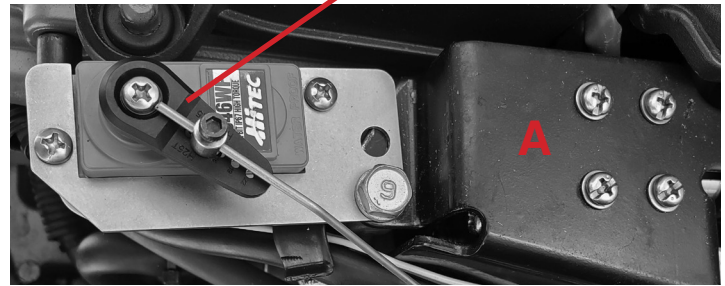
Fig 7: Servo horn position when iTroll is at Idle (0.0 %)
